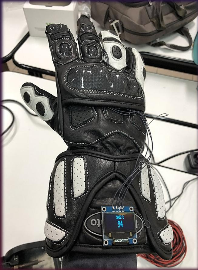
The project consists of a glove that enables us to monitor in real time the physical conditions of the pilot, showing us some vital parameters such as the heartbeat rhythm and the percentage of oxygen in the blood. The values identified by the sensor are displayed on a screen on the wrist.
